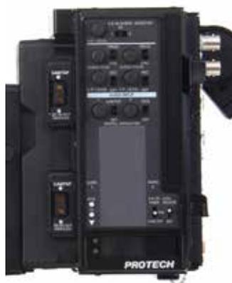
Specifications < 主な仕様 > ● INPUT/OUTPUT < 入力 / 出力 > SDI IN: BNCx1 12G/HD/SD, SDI OUT: BNCx1 Through Output, RET OUT/TC IN/TC OUT: BNCx1 each, REF OUT: BNCx1, Monitor IF: Mini 6P female x1, DC OUT: 120W (NS-X10) 170W (NS-X10GTS) ● FUNCTION < 機能 > TALLY Indicator: REDx1 H/L/OFF Switch, REMOTE: (1) 8P (2) 12P (L) 2.5 φ Mini Jack x1, LAN: RJ45, Intercom Headset: XLR 4P male x2 ● GENERAL < 一般 > Size (WxHxD): 201x163x110mm, Weight: 1.6 kg
