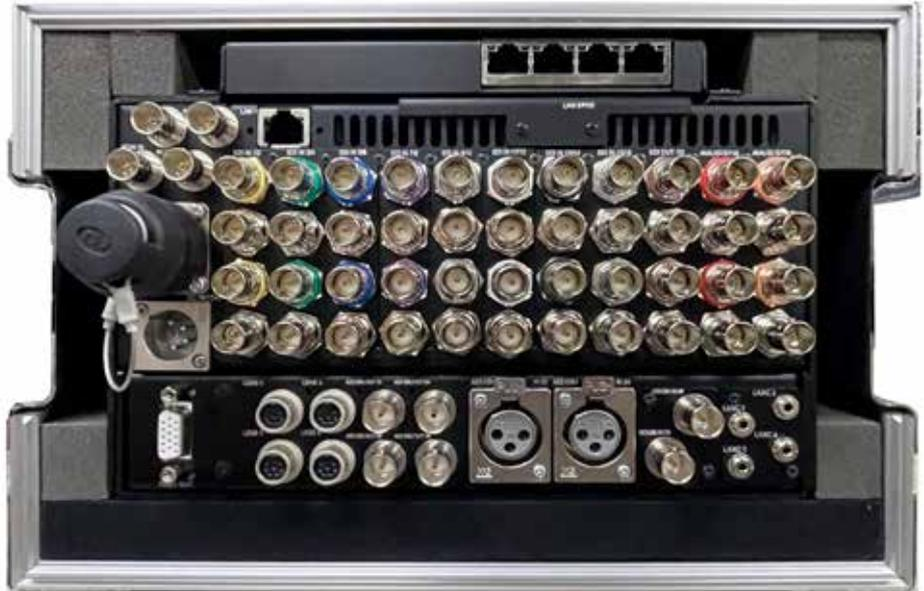
16ch 送り 6ch 受け / 大型光伝送装置 16ch feed 6ch receive / Large optical transmission equipment
