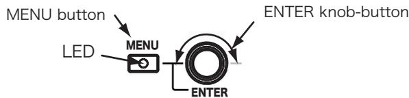
MENU button : Pressing the MENU button displays the MENU on the screen. Then the LED lights on.
