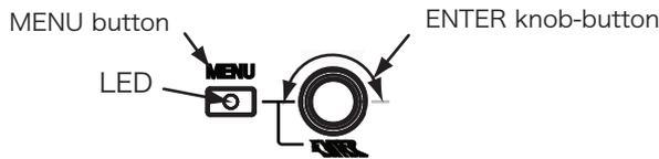
MENU button : Pressing the MENU button displays the MENU on the screen. Then the LED lights on. The cursor returns to the previous list by pressing this button while the LED lights on.
