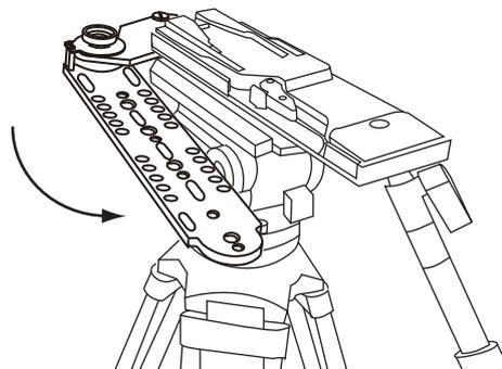
In case of using universal head, fit up the universal head to the bottom of the HD Monitor. And fix up the universal head and the HD Monitor onto the swing arm by w1/4 universal head screw.
